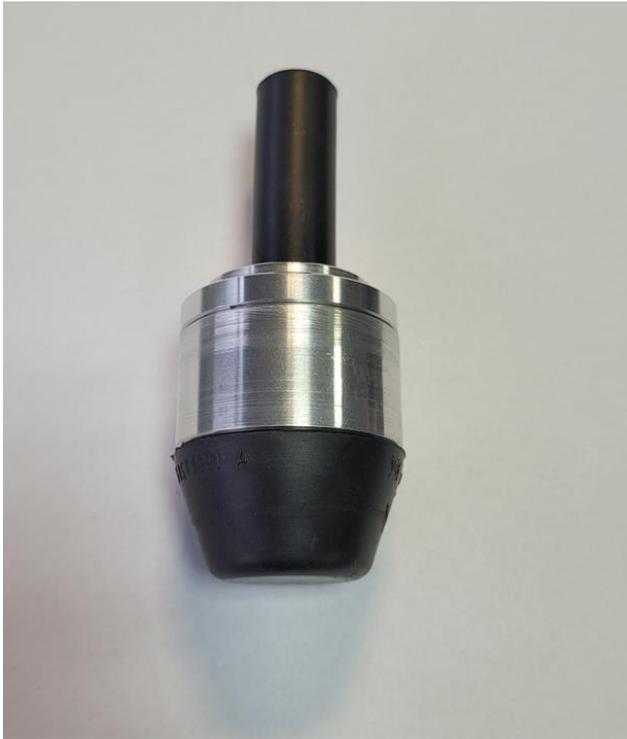
Then the original bump stop, which was dismantled, is clipped back into the lower part (Pos. 04), a little grease can be used for this if necessary.
