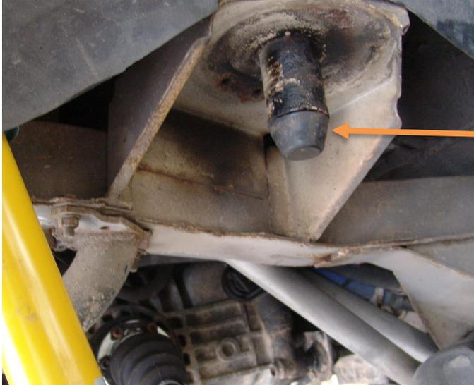
Series spring on the rear axle according to the workshop manual to be removed.
