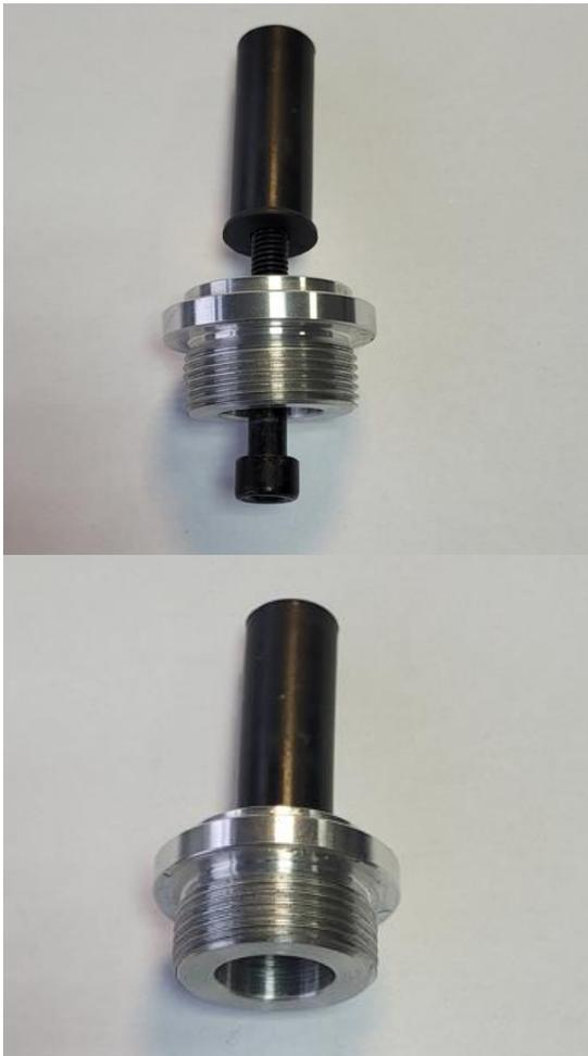
The upper part (Pos. 03) of the spring extension is pre-assembled with the supplied blind nut (Pos. 06) and the corresponding fastening screw (Pos. 05) as shown in the image.
